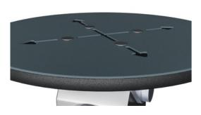
The ø414mm top plate is made from 15mm Ekogrip®, a 15mm PE plate with a 3mm top-layer of thermoplastic rubber with non-skid effect. The height is 217mm and the range of motion is +/- 90°, with a EPDM rubber stop at each end.
