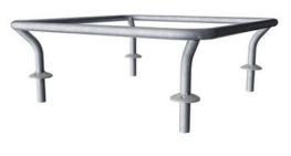
Handrail intended as grips during exercises are made of hot-dip galvanised steel ø38mm, a great diameter for a good grip and to support the wrist. The height of the handrail is 940mm from the top of the HPL plate. The distance between the rails is 900mm.
