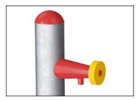
The integrated water tap open for water when pushed and stops when letting go. The water is supplied trough a pipe located inside the post with hose or pipe connection at the bottom of the post. The supply can either a loose hose or a permanent in-ground pluming.
