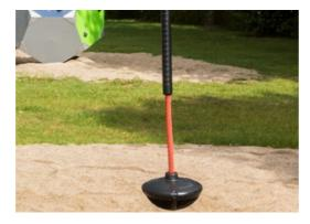
The specially designed seat is made from a stainless-steel insert covered with a soft layer of PUR rubber. The seat is impact tested to comply with global playground standards, and the rope has an ergonomic handhold of a 100cm long moulded on PUR rubber handle.
