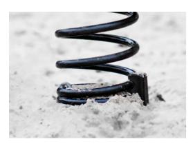
KOMPAN Springs are made of high quality spring steel according to EN10270. The springs are cleaned by phosphating before they are painted with an epoxy primer and a polyester powder coating as top finish. The springs are fixed by unique anti pinch fittings for maximum safety and long lifetime.
