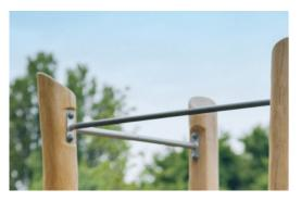
All bars intended for pull ups are made of solid,  $\emptyset 32\text{mm} \times 138 \text{ m}$ , hot dip galvanised, S235JR steel bars. This diameter gives the right grip for everyone.
