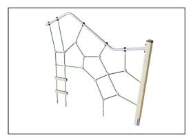
The rope nets are made of single braided 16 mm PES ropes. PES has high strength with excellent resistance to abrasion and UV radiation. The rope loops are assembled by aluminum connectors.
