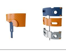
The climbing elements displayed are moulded in one piece with a minimum 5mm wall thickness. The climbing elements are made of recycable PE which has a high impact resistance across a wide temperature span which ensures vandal resistance in all locations.
