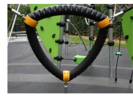
GALAXY climbing triangle with outer soft layer of PUR and corner brackets of moulded nylon (PA6). The core consist of a powder coated welded steel frame with integrated corner suspension points. Larger triangles are closed with an 18mm thick Ekogrip® panel that has a top-layer of rubber with a non-skid effect.
