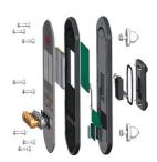
Front panels are made of UV-stabilized Polycarbonate. The UV-stabilization prevents the Transparent panels in being yellow over time and ensures the mechanical performances. The graphic prints are added by a unique multi-layer print process where the inner layer is the image and outer transparent layer functions as protection. The lacquer is water-based, and UV stabilized to prevent fading.
