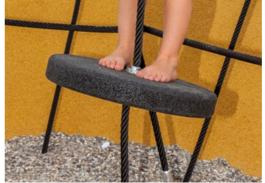
Fully coloured EPDM rubber discs with smooth surface. The moulded EPDM surrounds a hotdip galvanised steel core that ensures both the stability of the discs and durable fixtures to the rope.
