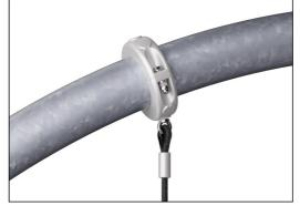
Corocord aluminium clamps are used as connectors between steel posts and rope. Two aluminium castings are bolted together. The height of the clamps is thus variable.
