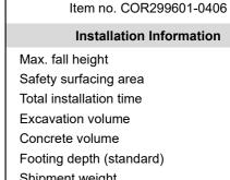
Installation Information 0 cm 26.2 m<sup>2</sup> 6.4 2.28 m<sup>3</sup> 1.27 m<sup>3</sup> 110 cm Shipment weight 343 kg In-ground Anchoring options
