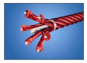
Corocord ropes with 19mm diameter or more are special 'Hercules' - type with galvanized sixstranded steel wires. Each strand is tightly wrapped with PES yarn. The ropes are connected by stainless steel S-Clamps which are pressed around the rope which results in a durable and vandalism solution.
