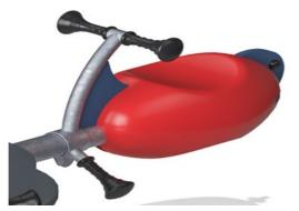
Handles and footrests are made with a molded PP insert and an outer layer of soft TPV rubber. The handles and footrests are attached to the pipe with a galvanized steel inlay to ensure strength and durability.
