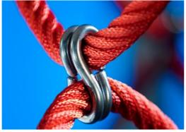
Designed to allow the typical function of rope play structures to move Corocord 'S' clamps are used as universal connections in Corocord products. 8mm stainless steel rods with rounded edges are pressed around the ropes with a special hydraulic press, making them the ideal connector. Our clamps are safe, durable and vandalism-proof.
