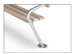
The steel surfaces are hot dip galvanized inside and outside with lead free zinc. The galvanization has excellent corrosion resistance in outdoor environments and require low maintenance. Painted steel parts are hot dip galvanized before powder coating.
