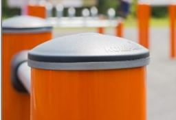
Post are made of Ø101.6 x 2mm, pregalvanized carbon steel and powder coated, a great protection to all conditions.
