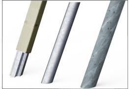
The A-Frame is available in three post-material options: Hot-dip galvanized 76mm steel, impregnated pine wood 95x95mm with hot dip galvanized steel footings, or 120mm TexMade™ posts.
