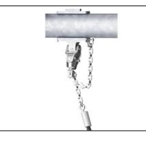
KOMPAN heavy duty designed swing hangers of stainless steel with anti-twist function. The hangers are attached to the cross beam on a welded bracket with two bolts, The bearings are embedded with silicone lubricant and needs no further lubrication.
