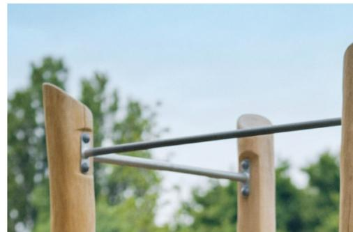
The pull up bar is made from Ø32 mm HDG steel bar. The bar is 1080mm wide and 2300mm above ground
