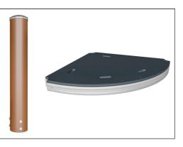
ELEMENTS decks are made of 17.8mm thick HPL supported by a unique designed aluminum frame with multiple attachment options by usage of aluminum connectors. The main posts are made of high quality pre-galvanised steel with powder coated top finish. Post tops are closed with caps of UV stabilised nylon (PA6). ELEMENTS products are available in three different colour combinations: classic blue & green, blossom orange & yellow, nature lime and green.
