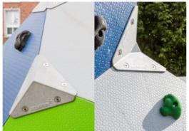
Die-casted corner brackets of high quality lead free aluminium. The corner brackets have nicely rounded edges and countersunk stainless steel screws. For hotter climates, the corner brackets can be supplied with optional powder coating which reduced the heat absorption of the brackets.
