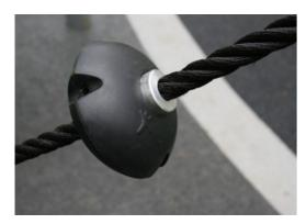
GALAXY ropes has six-stranded steel wires and a steel wire core. Each strand is tightly wrapped with PES yarn, which is melted onto each individual strand. The PES yarn is made of +95% Post-consumer materials and is inductively melted onto each strand to obtain excellent wear and tear resistance.
