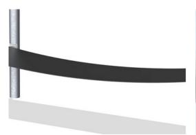
Membrane consisting of friction-proof rubberised material of conveyor belt quality with excellent UV resistance. Tested and compliant with REACH requirements for PAH. Embedded are two layers of galvanised steel wire armouring, making the membrane extremely hardwearing and vandalism resistant. Core and outer layers result in a total thickness of 10mm.
