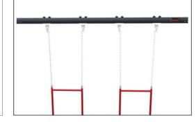
Note: As the You & Me seat uses heavy duty swing hangers the seat can not be fitted onto swings with traditional swing hangers. In such cases a new crossbeam with heavy duty hangers must be installed.
