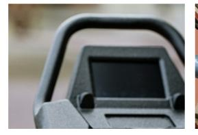
The handle bars is designed with multiple hand positions to accommodate different postures and riding styles. It is a casted Aluminium part with Polyurea coating for good grip and insulation.
