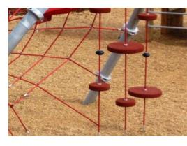
Corocord 16mm ropes of UV-stabilized PES rope strands with inner steel cable reinforcement. The polyester yarn is made from +95% post-consumer materials and is inductively melted onto each strand. The ropes are highly wear-and vandalism-resistant and can be replaced at site if needed.
