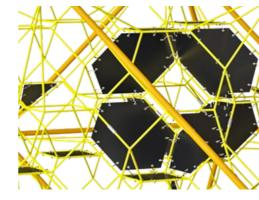
Corocord membranes consist of friction-proof rubberised material of conveyor belt quality with excellent UV resistance. Tested and compliant with REACH requirements for PAH. Embedded is a four-layered armouring made of woven polyester. The armouring and the two surface layers result in a total thickness of 7.5 mm.
