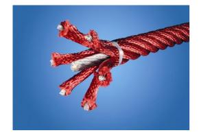
Corocord ropes with 19mm+ diameter are known as a 'Hercules' rope type which is formed from galvanised six-stranded steel wires. Each strand is tightly wrapped with PES yarn, which is melted onto each individual strand. Ropes are highly wear-and vandalism-resistant and can be easily replaced on-site if needed.
