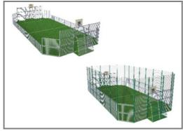
Post length above ground can differ from 1, 2, 3 & 5m high. In the surface mount solution, the footing is 200 x 200 x 10mm. As an in-ground solutions, the post will go 45cm below ground for side panels and 90cm for goal panels.
