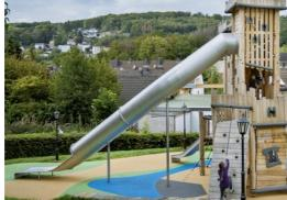
Curved and straight stainless-steel tunnel slides are supported by multiple steel rods to a centre steel post. KOMPAN tunnel slides have been designed with a perfect curve and inclination for a playful ride.
