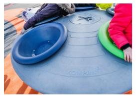
The Multispinner grey base is made of recyclable PE made from 33% post-consumer Materials. The base is moulded in one piece with integrated metal thread bushings and water drain holes to ensure high durability in all climates around the world. Each bowl is mounted separately into the base.
