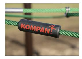
Ropes of UV-stabilized PES rope strands with inner steel cable reinforcement. The polyester varn is made of +95% Post-consumer materials and is inductively melted onto each strand to obtain excellent wear and tear resistance.
