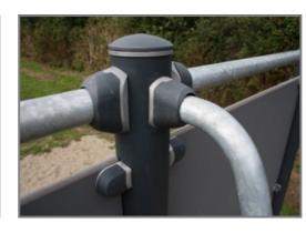
The connectors are made of die-cast aluminium, specially alloyed for the outdoor environments and heavy usage. The screws attaching the connectors are stainless steel and protected by zinc washers.
