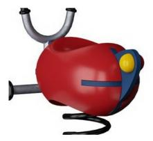
The seat is made of recyclable PE and moulded in one piece with a minimum 5mm wall thickness. PE has high impact resistance across a wide temperature span which ensures vandal resistance in all locations.
