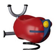
The seat is made of recyclable PE and moulded in one piece with a minimum 5mm wall thickness. PE has high impact resistance across a wide temperature span which ensures vandal resistance in all locations.
