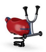
KOMPAN's springs are manufactured from highquality spring steel. The springs are cleaned by phosphating before being painted with epoxy primer and polyester powder coating. The springs are fixed by unique anti-pinch fittings for maximum safety and longevity.
