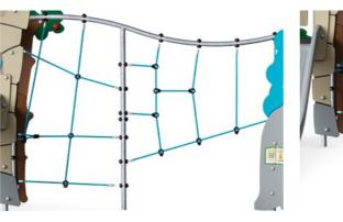
Climbing nets are made of UV-stabilised PP rope with inner steel cable reinforcement. The rope is induction treated to obtain maximum fixation between steel and rope which provides excellent wear and tear resistance. All rope connectors are made of 100% recyclable PA material. The steel surfaces are hot dip galvanised inside and outside with lead free zinc. The galvanisation has excellent corrosion resistance in outside environments and requires low maintenance.
