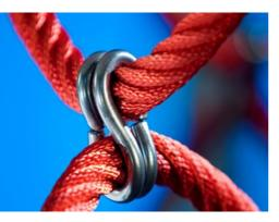
Designed to allow the typical function of rope play structures to move Corocord 'S' clamps are used as universal connections in Corocord products. 8mm stainless steel rods with rounded edges are pressed around the ropes with a special hydraulic press, making them the ideal connector. Our clamps are safe, durable and vandalism-proof.
