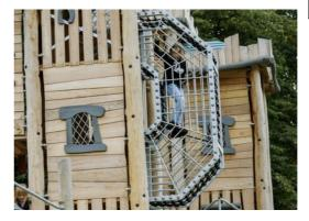
The wire frame tunnel is made of hot dip galvanised high quality steel. Corocord 16mm ropes of UV-stabilized PES rope strands with inner steel cable reinforcement. The polyester yarn is made from +95% post-consumer materials and is inductively melted onto each strand. The ropes are highly wear-and vandalism-resistant and can be replaced at site if needed
