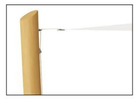
The rope is attached to the Robinia post by a stainless-steel eyebolt and tightened by a nylon bracket with wedge track. The system ensures the sail is easy to set-up, tighten and take down again.
