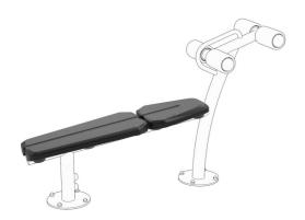
The seat and back support are made of Polyurethane Rubber (PUR) and have an electro-galvanized steel insert plate that connects the seat to the steel frame. The seat and the back support are positioned under an 8degree angle for the correct ergonomics. The back support has a groove to relieve the spine, accommodating a comfortable seating position, another benefit is that it drains water easily.
