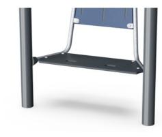
The steps are made of High Pressure Laminate HPL with a thickness 17,8mm and non skid surface texture according to EN 438-6. KOMPAN HPL has high wearing strength to ensure long lifetime in all climates.
