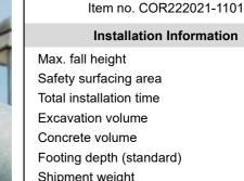
Installation Information 230 cm Safety surfacing area 123.1 m<sup>2</sup> Total installation time 11.5 Excavation volume 9.33 m<sup>3</sup> 5.94 m<sup>3</sup> Footing depth (standard) 110 cm Shipment weight 547 kg In-ground Anchoring options
