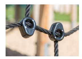
Nets and ropes are made of UV-stabilised PA with inner steel cable reinforcement. The rope is induction treated to create a strong connection between steel and rope, which leads to durable weather resistance. The Robinia wood can be supplied as untreated raw wood or painted with a brown coloured transparent pigment that maintains the golden wood colour of the wood.
