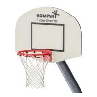
The basketball hoop is made from hot dipped galvanized steel with a powder coated finish. The net is made from Ø4 chain links made from s235 Galvanized steel or stainless-steel chains which meet the requirements in ISO1434-ISO1435 and DIN766. The chains have a circumference of  $\sim$ Ø30cm at the bottom and  $\sim$ Ø50cm at the top.
