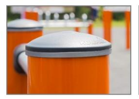
The post is made of Ø101.6 x 2mm, pregalvanised carbon steel and powder coated which is a great protection solution for all climate conditions.
