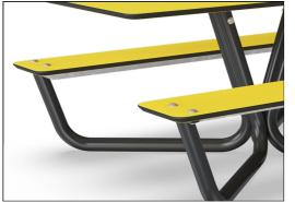
All boards are made of High Pressure Laminate HPL with a thickness of 17.8mm according to EN 438-6 and has a nonskid surface texture. The multilayer construction makes the boards durable and suitable for outdoor use with a high UV stability and high resistance to impacts, scratches, fire, water and humidity.
