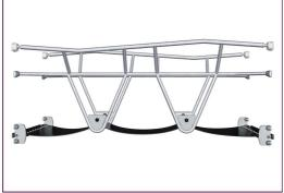
ELEMENTS rubber membranes are conveyer belt made of layers of rubber mixed of natural rubber and SBR rubber, and embedded with layers of armouring made of woven PE and PA. The thickness 8mm ensures high durability in any environment.
