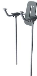
The frame of the leg lift is made from  $\text{Ø}38 \times 2\text{mm}$  HDG steel tube. The support plates are made from 15mm Ekogrip®, a 15 mm PE plate with a 3 mm top-layer of thermoplastic rubber with non-skid effect. The arm supports are 110 x 195mm, 580mm apart, and 1315mm above ground. The back support is 335 x 500mm. The opening in the back is 30 x 350mm.
