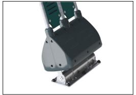
The rocking movement back and forth is controlled by a heavy duty scaled double rubber torsion spring element. The rubber element ensures a safe movement and reduces speed towards the tower platforms. The base cover of molded PE material with high impact resistance.
