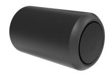
The rotating rollers are  $\emptyset$  110mm and made from PUR (Polyurethane Rubber, compact foam). The rollers have a steel insert that is electro galvanized. They provide support and ensure a comfortable position.
