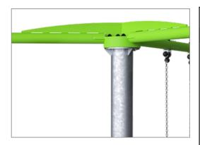
Center post is hot-dip galvanised in dimension Ø159 x 4 mm. Horizontal beams are hot-dip galvanised and powder coated in dimension of Ø76,1 x 3,6 mm.
