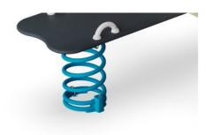
KOMPAN's springs are manufactured from highquality spring steel. The springs are cleaned by phosphating before being painted with epoxy primer and polyester powder coating. The springs are fixed by unique anti-pinch fittings for maximum safety and longevity.
