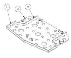
A 5 mm hot-dip galvanized carbon steel plate must is molded inside the SBR to offer optimal stability and optimize the mounting of the step
